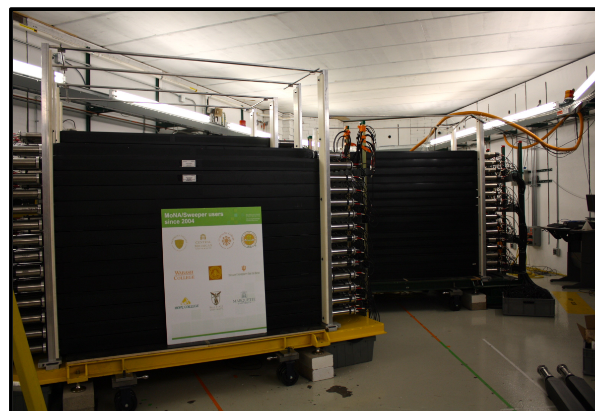
MoNA and LISA scintillator arrays, N2 vault at NSCL
